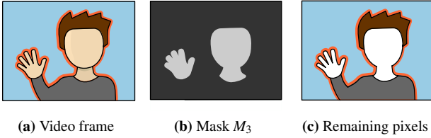
Figure 6: Partial removal of foreground using skin color detection (● = environment, ● = virtual bg). Image regions with human skin color are removed.
